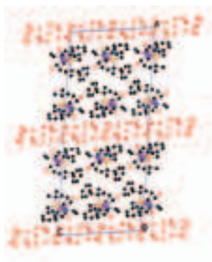
Unit cell of a water-activated ruthenium pincer complex
