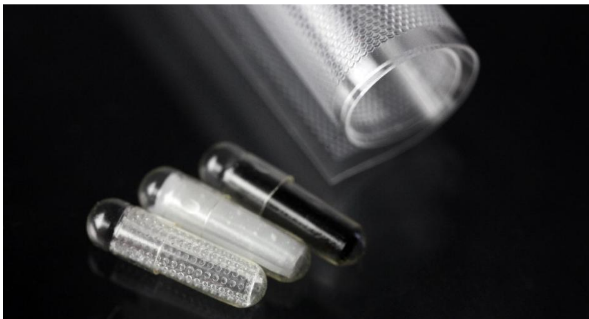
Foils and foils loaded into gelatine capsules for oral delivery. Source: CORDIS, FREJA project.
