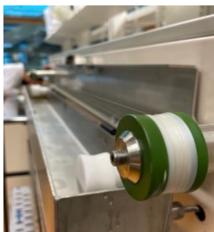
1: Collection of multifilament artificial spider silk fibres ( ArtSilkTex ); 2: Biomimetic artificial spider silk fibres spun within the ARTSILK project. Source: CORDIS.
