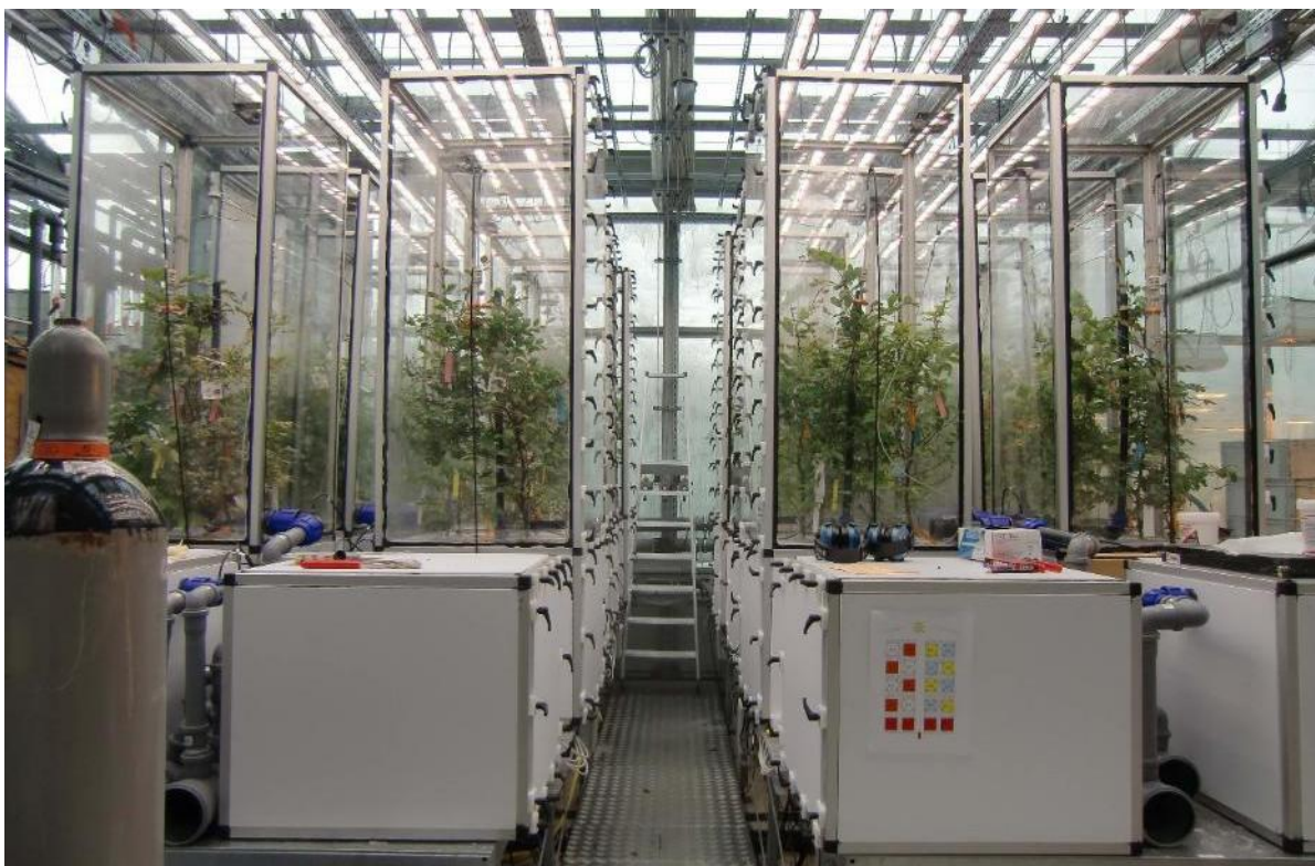
QUINCY mesocosm experiment with 16 tree chambers (back) and 4 soil control chambers (front). Source: CORDIS.
